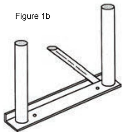
A continuous bearing plate joining the two posts
