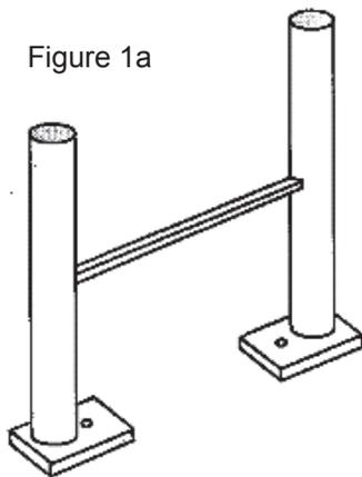
Bearing plates are placed under each post
